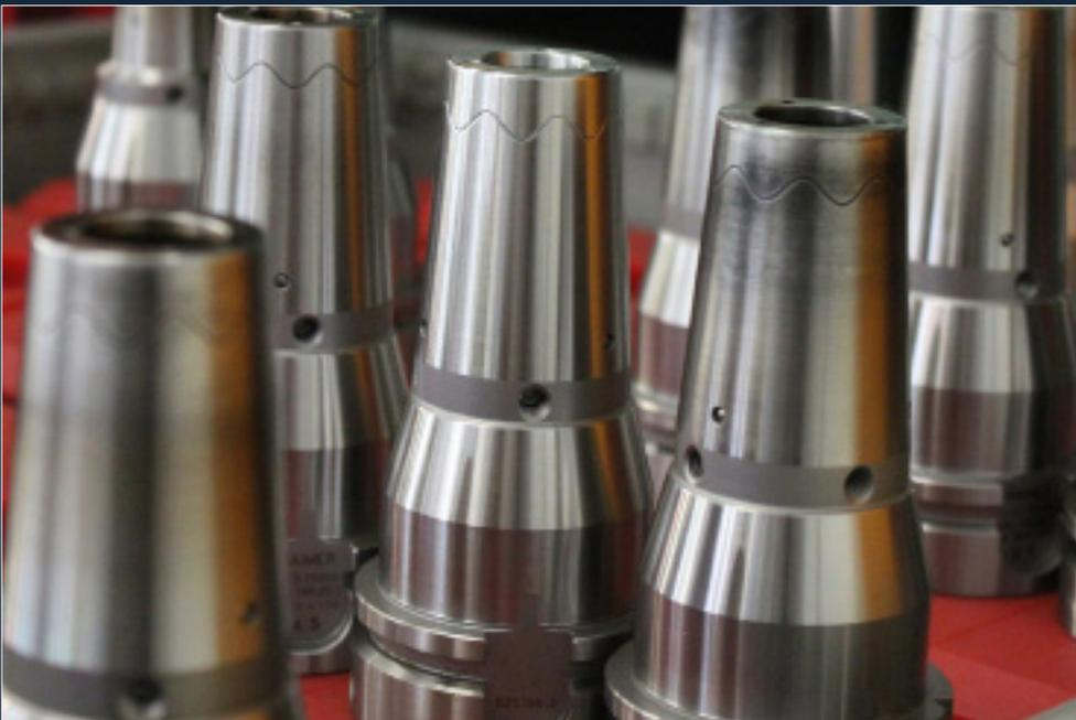
DGW chose Haimer holders for the superiority and durability of the power-shrink system. Power-shrink keeps runout to an absolute minimum with even our smallest drills and creates perfect seals for high-pressure through-spindle coolant.
