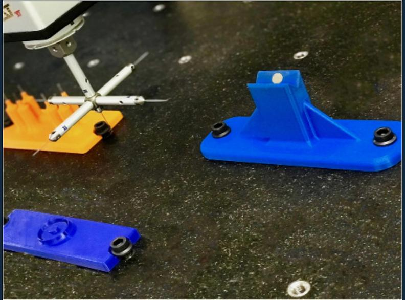
**Our alternative to these wasteful and expensive practices is 3D printing. Our Stratasys Fortus 250MC is capable of build volumes of up to 1200 cubic inches and the accuracy of .007" layer thickness. Unlike traditional machining, jobs are typically processed and running within 30 minutes.**
